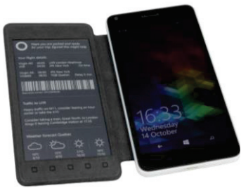
Figure 1: Our working prototype Display Cover is fully integrated with a Lumia 640 smartphone. The cover is less than 3mm thick in total, making it comparable to a regular protective cover.
